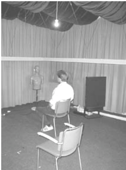
Figure 3: Experiment set-up with the two listening positions (chairs). The subject is sitting at position 2, the empty chair is listening position 1.
