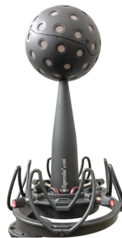
Figure 17: EM64 Eigenmike® (by MH-Acoustics)
