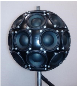
Figure 5: Prototype spherical array loudspeaker [1]
