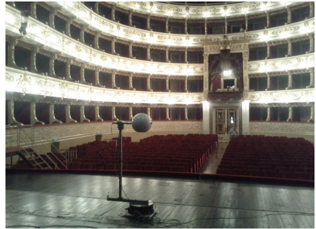
Figure 7: The single sphere loudspeaker on the two-axes turntable, inside Teatro Regio of Parma
