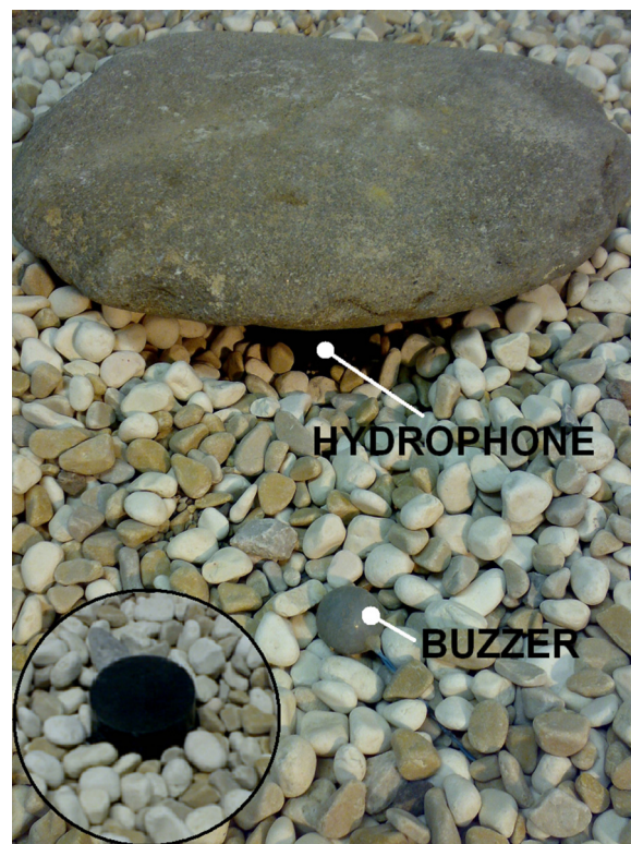
FIG. 1. (Color online) Picture of the position of the hydrophone (GLG 9190) and the buzzer during the “SOURCE OUT” measurement of a flat stone (weight: 580 g). Inset: The hydrophone shown without the stone above. All photos are taken in laboratory for convenience.
