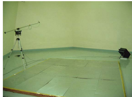
Fig. 7. Sound absorption test in an anechoic room.
