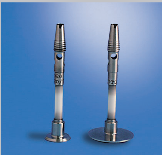
High-temperature geometries with ceramic shaft at different diameters
