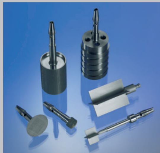
Selection of special measuring geometries with serrated surfaces to prevent slippage, with helical groovings to prevent sedimentation, vane rotors and rotors with glass covers
