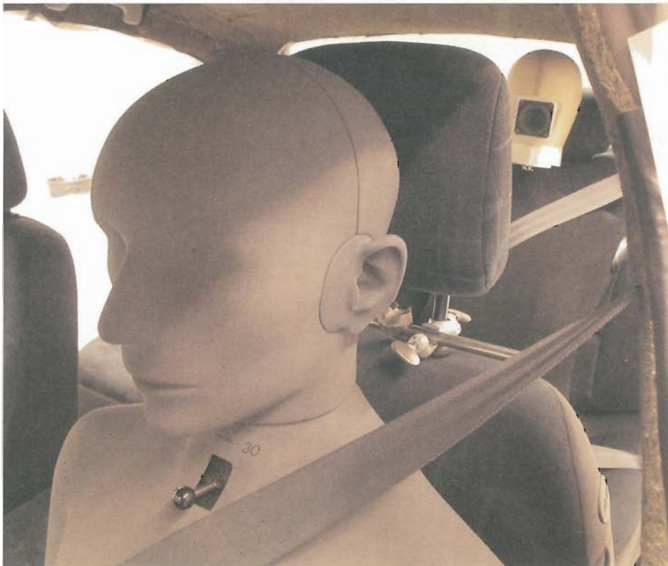
Fig. 7 STI Measurement set-up
