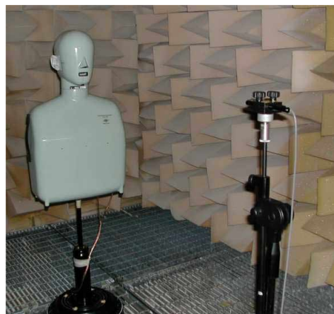
Figure 5 : Brüel & Kjær mouth simulator type 4230 on rotating table.
