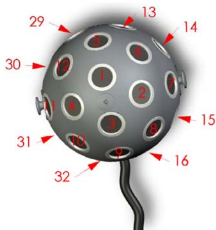
Figure 8: positions of the 32 capsules of the Eigenmike™.
