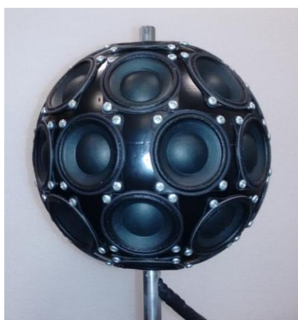
Figure 10 – the 32-speakers array
