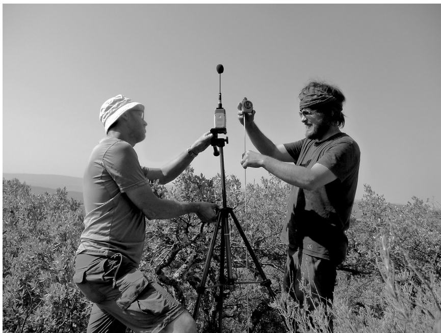
Fig. 2. The modified Zoom H2 digital recorder connected to the Brahma™ microphone during the Impulse Response (IR) measurement in the adjacent area of the shelter S8 at Baume Brune.
